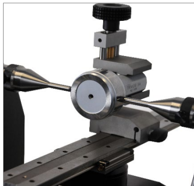
Checking of plug gauges and pin gauges (max. \varnothing 100mm/4", length 280mm/11") (TULM6/L0.5, LABC15)
