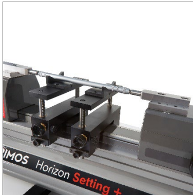
Setting of 2-point internal measuring equipment (TELMA7)
