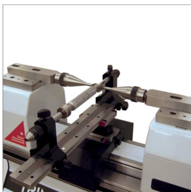
Etalonnage de tampons filetés (HPA-1, TEL6, 3P/0.17-3.2 /S6.5, LABC-15)
