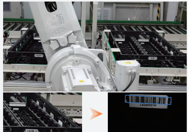
Dirty wear and low contrast barcode reading on logistics line pallet
