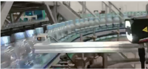
Package labeling guide ultra-high speed inspection
