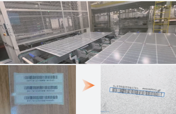
Distorted code reading on covered PV module
