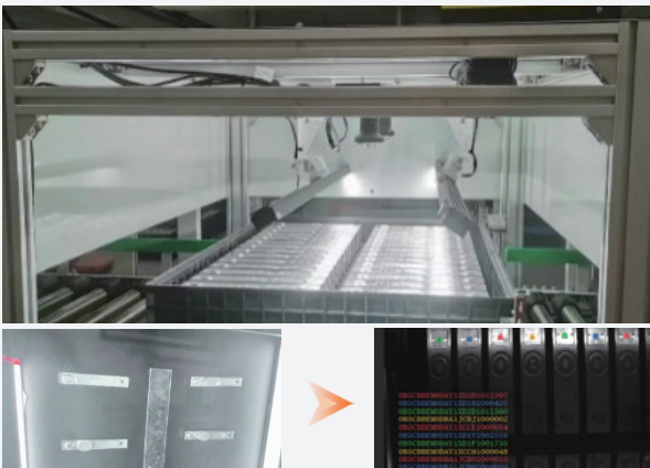
Battery top cover reflective small code batch reading in turnover boxes
