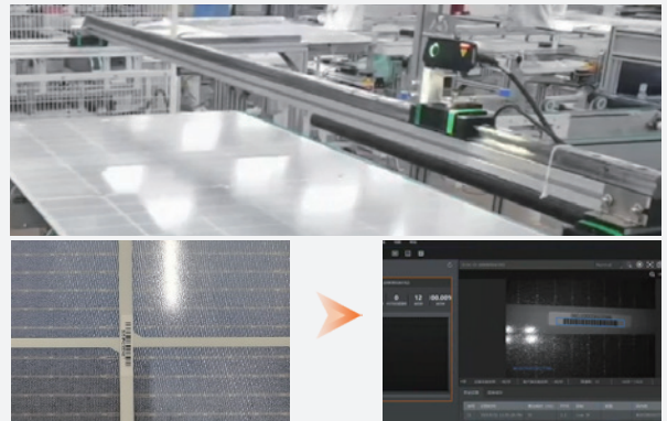
Code 128 reading on PV module backboard
