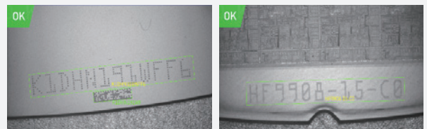
Silicon wafer SEMI font recognition
