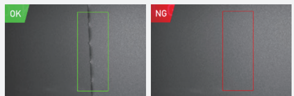
Lithium battery tab zigzag detection
