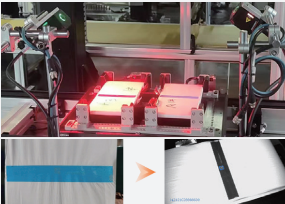
Battery cell code reading on blue tape
