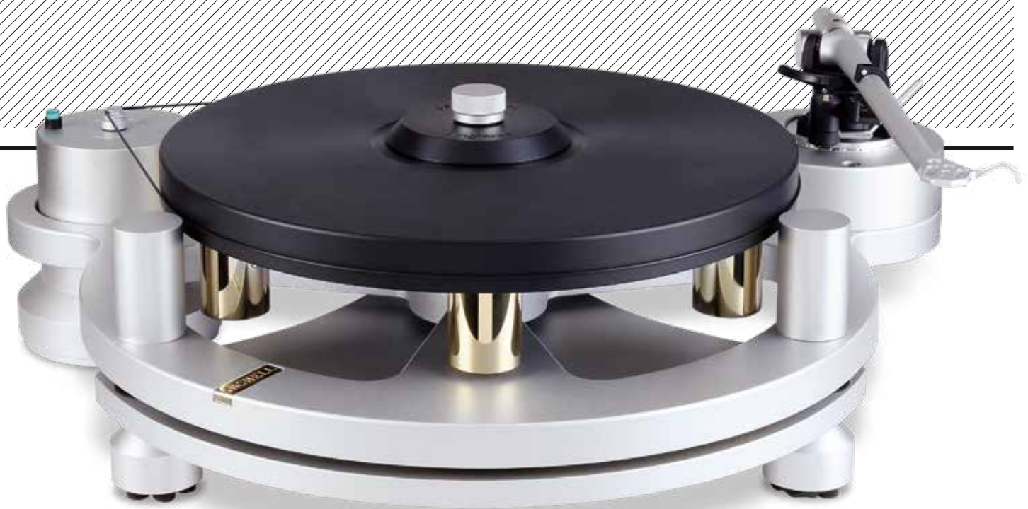
ABOVE: A DC motor drives the Delrin platter via a continuous rubber belt, the six underslung gold-plated brass weights adding peripheral mass. Our deck was fitted with the TecnoArm 2
