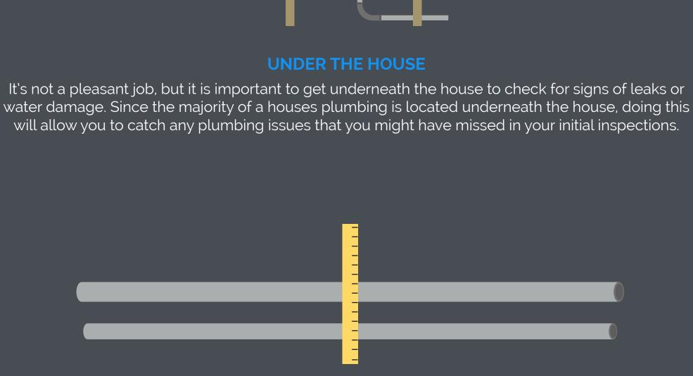
lower and could increase the potential for damage in the future. In most cases, you will want the pipes to be 3/4" from the source of water to the home, and 1/2" or larger from sinks and taps.
