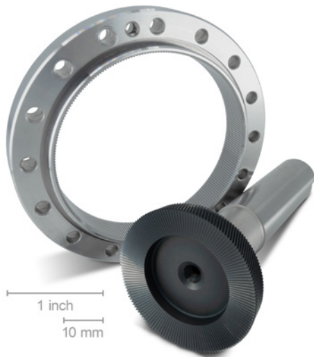
Example 1—Conical, a solid-carbide tool with AICroNite Pro coating for power skiving of strain wave gears in robotic drives. Cutting time is just 0.6 min—much faster than conventional shaping.
