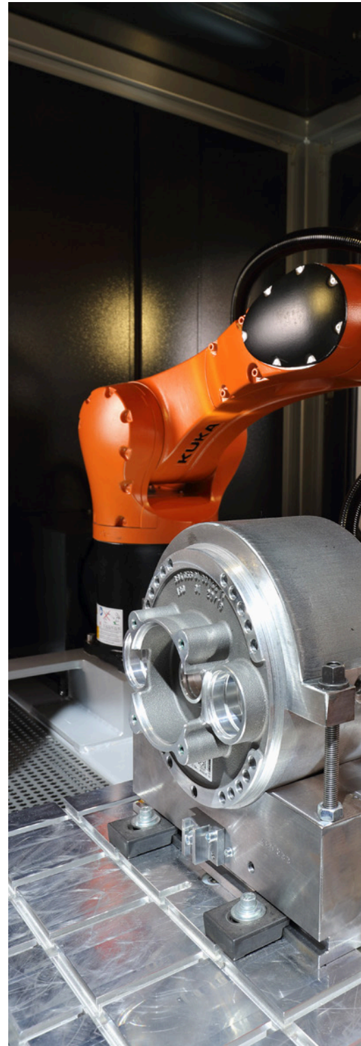
The KUKA KR Agilus is used to deburr a gear housing.
