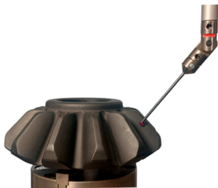
Figure 9—CMM evaluation and inspection report.
