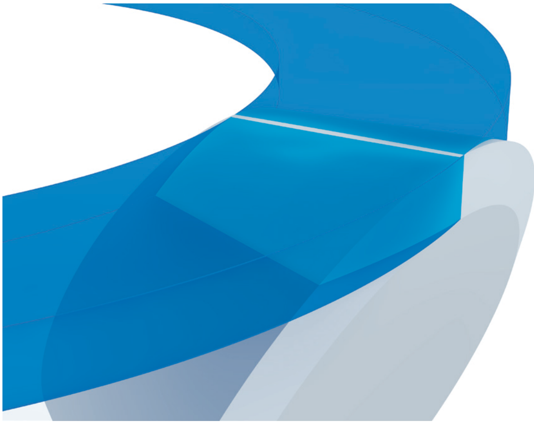
Figure 6—Hypoid pinion and its crown gear—Method 1 with the intrinsic pitch cone.
