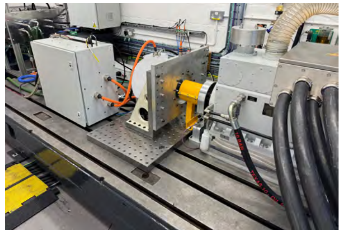
Test cells measure realistic failure modes that focus on operational consequences of the drive systems.
