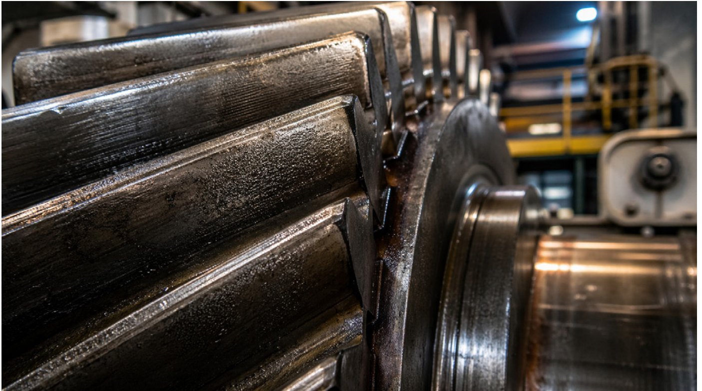
Figure 1—Early-stage surface fatigue and distress on a heavy-duty gear tooth flank. Surface damage may progress well before catastrophic failure becomes visible. (All Images: Pamilanga Ltd.)
