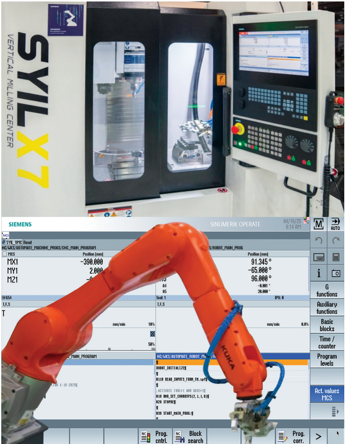
Figure 1—Displayed here are the Syil machine tool and Kuka robot interacting, with all motions run on the Sinumerik RunMyRobot/Handling application directly in the control. (All images: Siemens)
