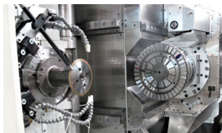
Figure 13—Grinding of a Coniflex coupling with a CBN-grinding wheel.
