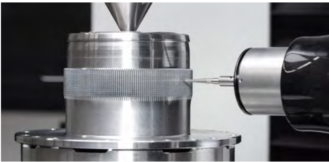
Inspection of external strain wave gear on the 175GMS nano Gear Metrology System.
