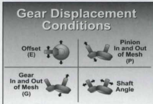
Figure 4—Gear displacement conditions. time-consuming and costly process, it was just the way it had to be done—or it was until new computer-based technologies for gear development became available.
