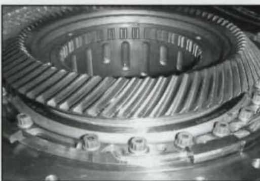
Figure 12—A spiral bevel gear after running in the aircraft jet engine for 75 hours. Contact pattern is exactly as predicted.
