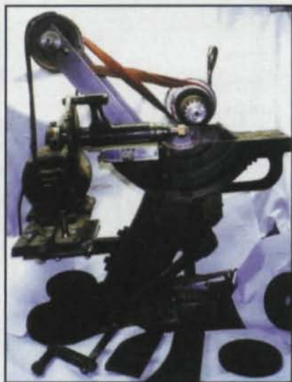
An antique, hand-operated gear-cutting machine manufactured by Sloan, Chace & Co.
