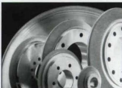
Gleason Cutting Tools Corp. expanded its production capacity for high precision, CBN-plated wheels used for external and internal, straight and helical, parallel and bevel gear grinding.
