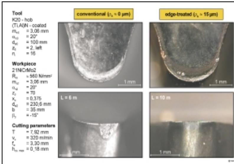
Figure 7—Wear behavior depending on the edge treatment.
