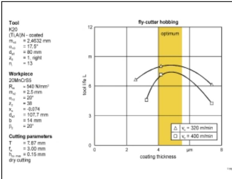
Figure 3—Tool life depending on the coating thickness.
