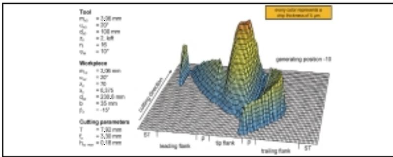
Figure 9—3-D illustration of a simulated chip's geometry.
