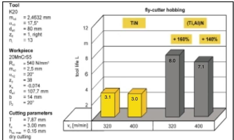
Figure 2—Advantages of (Ti,Al)N coatings in dry hobbing.
