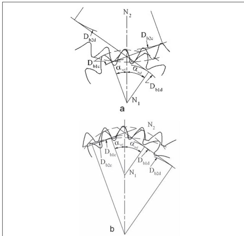
Figure 4—Asymmetric gear mesh; a—external gearing; b—internal gearing;  $\alpha_w$ —operating pressure angle;  $D_{b1,2}$ —operating pitch circle diameters; subscripts “1” and “2” are for the mating pinion and the gear.
