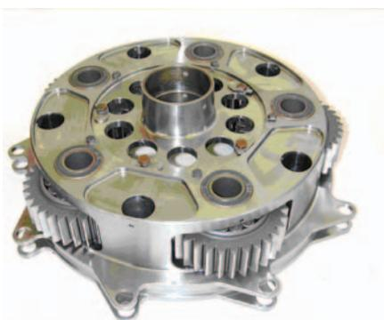
Figure 9—Second-stage carrier assembly.
