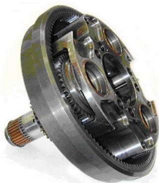
Figure 7—First-stage carrier and ring gear assembly.
