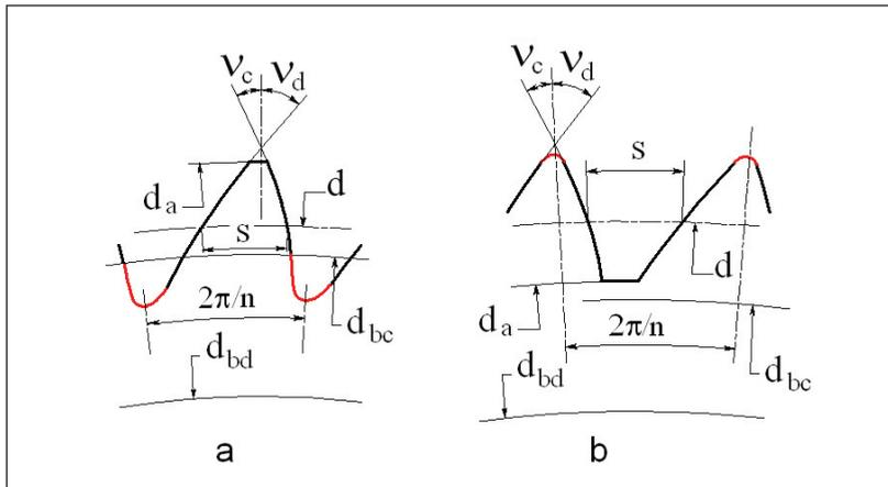
Figure 3—Asymmetric tooth profile (the fillet portion is red); a—external tooth; b—internal tooth;  $d_a$ —tooth tip circle diameter;  $d_b$ —base circle diameter;  $d$ —reference circle diameter;  $S$ —circular tooth thickness at the reference diameter;  $v$ —involute intersection profile angle; subscripts “d” and “c” are for the drive and coast flanks of the asymmetric tooth.
