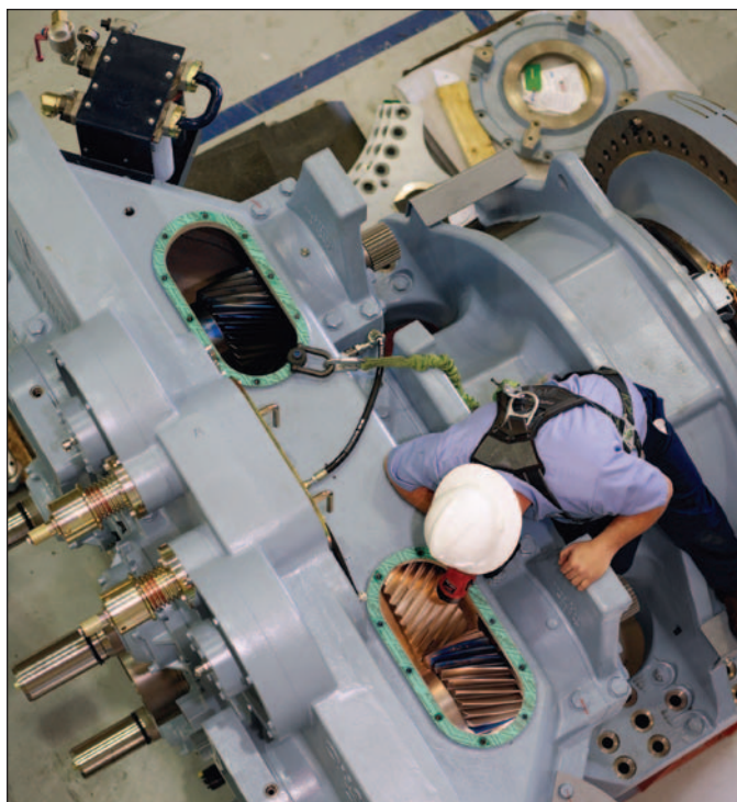
The gearboxes and gears used in today’s wind turbines are some of the most technologically advanced in the world. Finding skilled designers and workers to make them continues to be a problem for the industry. Photo courtesy of Clipper Windpower.
