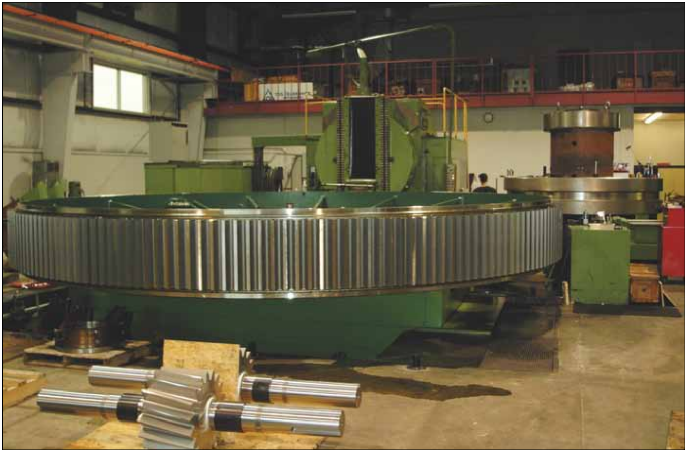
A ring gear for a mining operation gets the final touches at Havlik International before shipping out to the customer (courtesy of Havlik).
