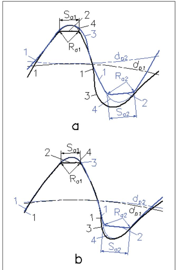
**Figure 7—The fillet profile construction. a: external gears; b: internal gearing; 1: involute profiles; 2: tooth tip lands; 3: fillet profiles; 4: ellipsis arcs that are used to generate the fillet profiles.**
