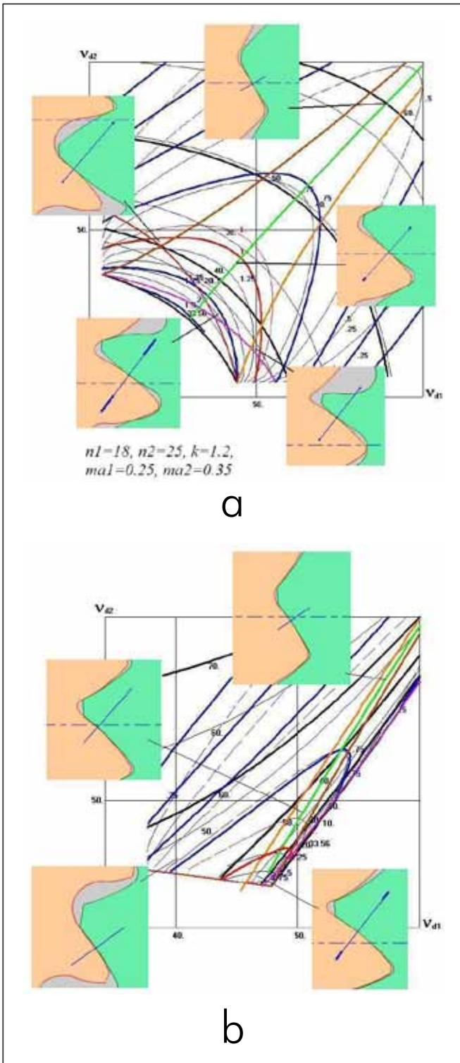
**Figure 6—Area of existence for the asymmetric pinion and gear with:  $n_1 = 18$  and  $n_2 = 25$ ;  $m_{a1} = 0.25$  and  $m_{a2} = 0.35$ ; and  $k = 1.2$ . a: for external gearing; b: internal gearing. The isograms related to the drive flank meshes are thick, the isograms related to the coast flank meshes are thin.**
