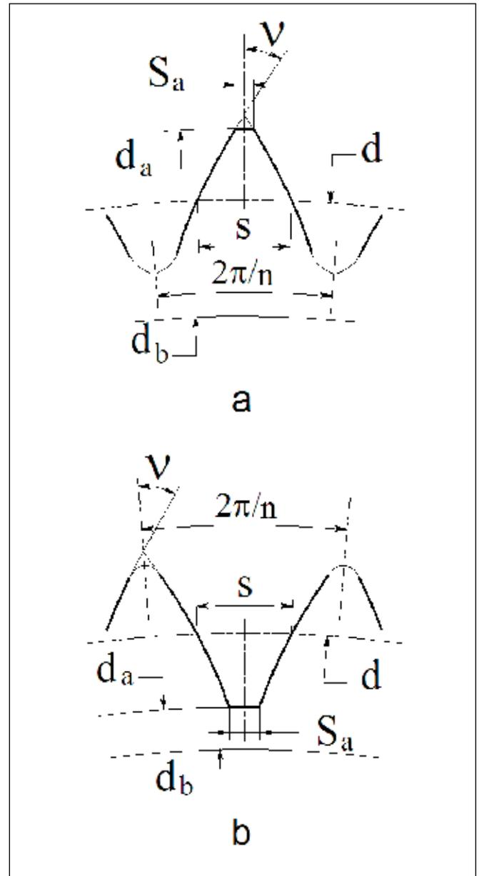
Figure 2—Tooth profile. a: external tooth; b: internal tooth;  $n$ : number of teeth;  $d_a$ : tooth tip circle diameter;  $d_b$ : base circle diameter;  $d$ : reference circle diameter;  $S$ : circular tooth thickness at the reference diameter;  $\nu$ : involute intersection profile angle;  $S_a$ : circular tooth thickness at the tooth tip diameter.
