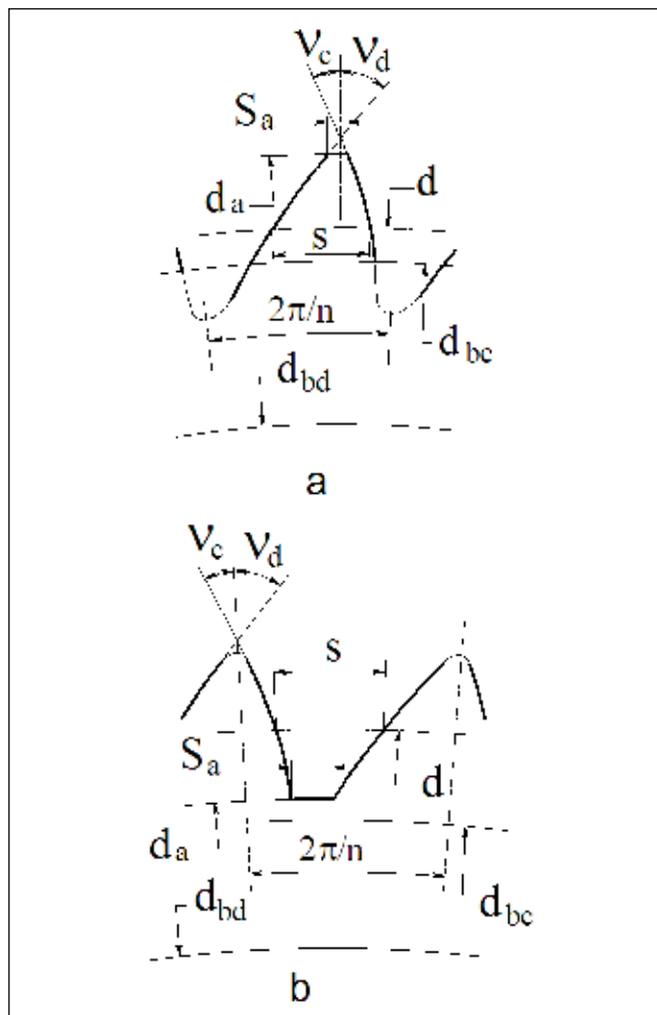
Figure 5—Asymmetric tooth profile (fillet portion red); a: external tooth; b: internal tooth;  $d_a$ : tooth tip circle diameter;  $d_b$ : base circle diameter;  $d$ : reference circle diameter;  $S$ : circular tooth thickness at the reference diameter;  $v$ : involute intersection profile angle;  $S_a$ : circular tooth thickness at the tooth tip diameter; subscripts "d" and "c" are for the drive and coast flanks of the asymmetric tooth.
