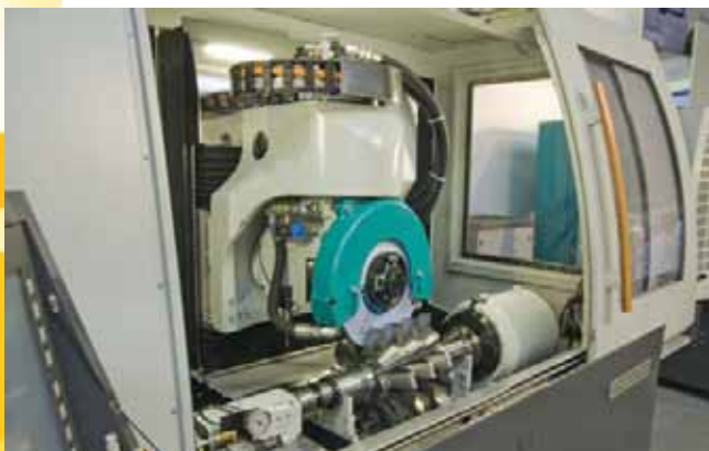
Schneeberger Large End Hob Grinder Up to 20" Diameter H obs with 20" Wheels. 52 Hp (100%) Power Plant.
