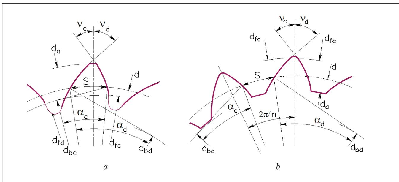
**Figure 1—Gear tooth profile: a = external gear; b = internal gear;  $d_a$  = tooth tip circle diameter;  $d_b$  = base circle diameter;  $d_f$  = form circle diameter;  $d$  = reference circle diameter;  $S$  = circular tooth thickness at the reference diameter;  $\alpha$  = involute profile (or pressure) angle at the reference diameter;  $v$  = involute intersection angle;  $n$  = number of teeth; subscripts “d” and “c” are for the drive and coast flanks of the asymmetric tooth.**
