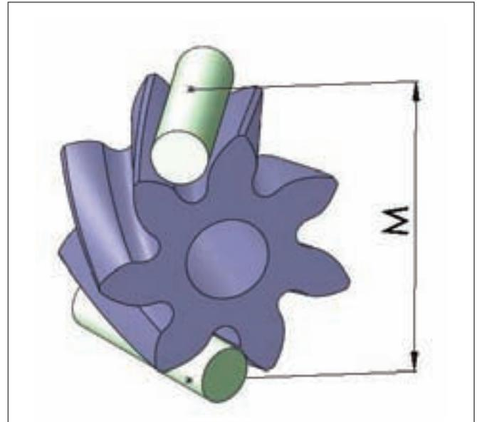
Figure 8—Measurement over pins of the external helical gear with odd number of teeth.
