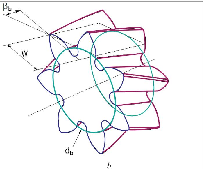
Figure 9—Span measurement; *a* = spur gear; *b* = helical gear.
