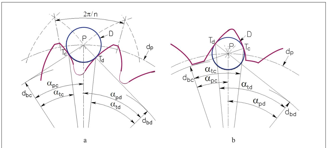
**Figure 2—Ball or pin position: a = external gear; b = internal gear; D = ball or pin diameter; P = center of the ball or pin;  $\alpha_{pd}$  and  $\alpha_{pc}$  = involute profile angles at the center of the ball or pin;  $d_p$  = ball or pin center location diameter;  $T_d$  and  $T_c$  = contact points of the ball or pin with the tooth drive and coast tooth flanks;  $\alpha_{td}$  and  $\alpha_{tc}$  = involute profile angles at the contact points.**
