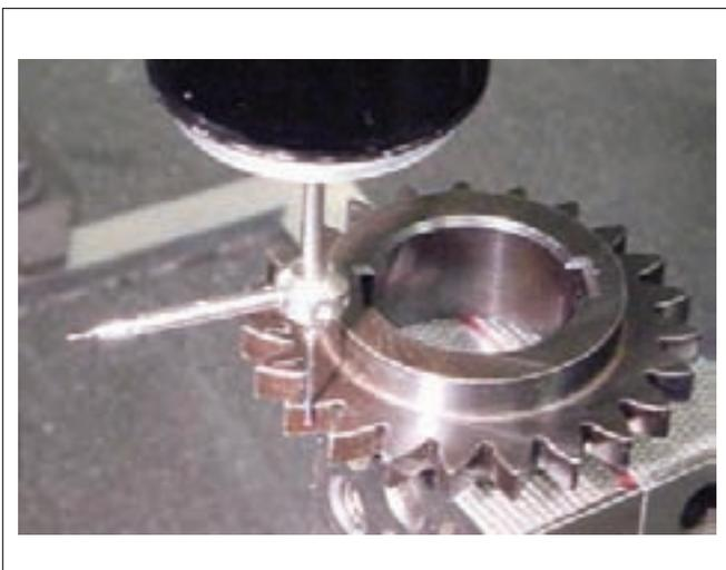
Figure 10—CMM measurement of asymmetric gear.
