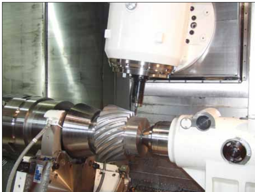
Through simultaneous five-axis machining, Mazak's Integrex e-670H II can produce complex shaft workpieces containing tapered holes, blisks and spiral bevel gears in a single setup (courtesy of Mazak).
