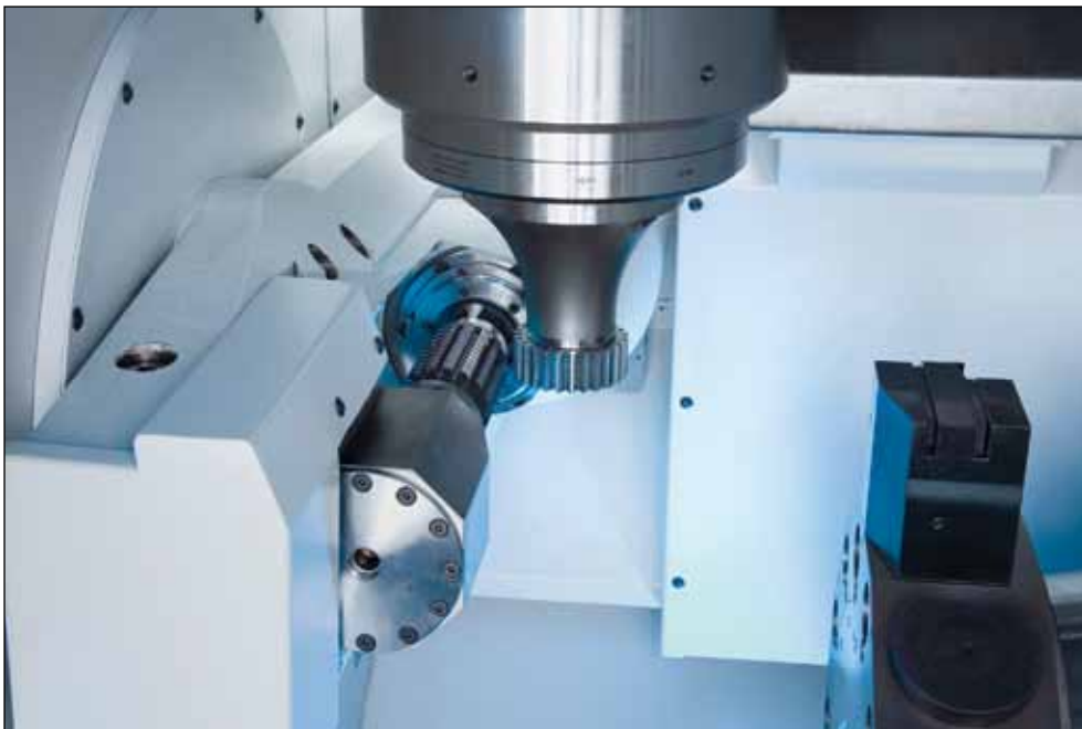
The design of EMAG's VSC 400 DUO WF multifunctional machine is based on the pick-up principle of the EMAG single-spindle turning machine and features both gear turning and gear hobbing operations (courtesy of EMAG).
