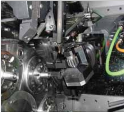
For the machining of gears, a module two or smaller fits the capabilities at Index and Traub (courtesy of Index).
