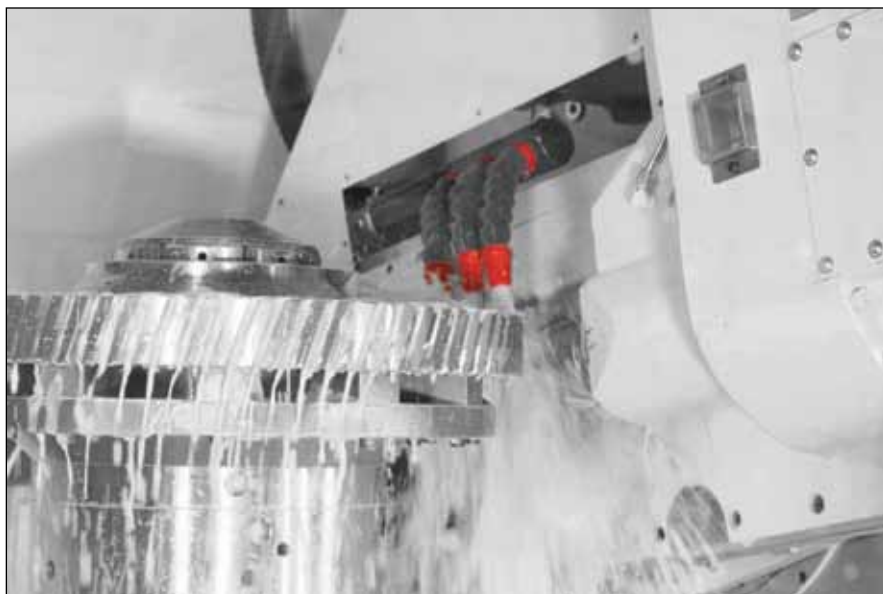
Various gear operations can be performed on MAG's line of vertical turning centers (courtesy of MAG).
