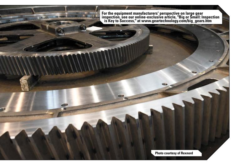
quality, simply because casting such a heavy part (more than 20 tons a segment, finished weight) has nothing to do with casting a 3-ton segment."
