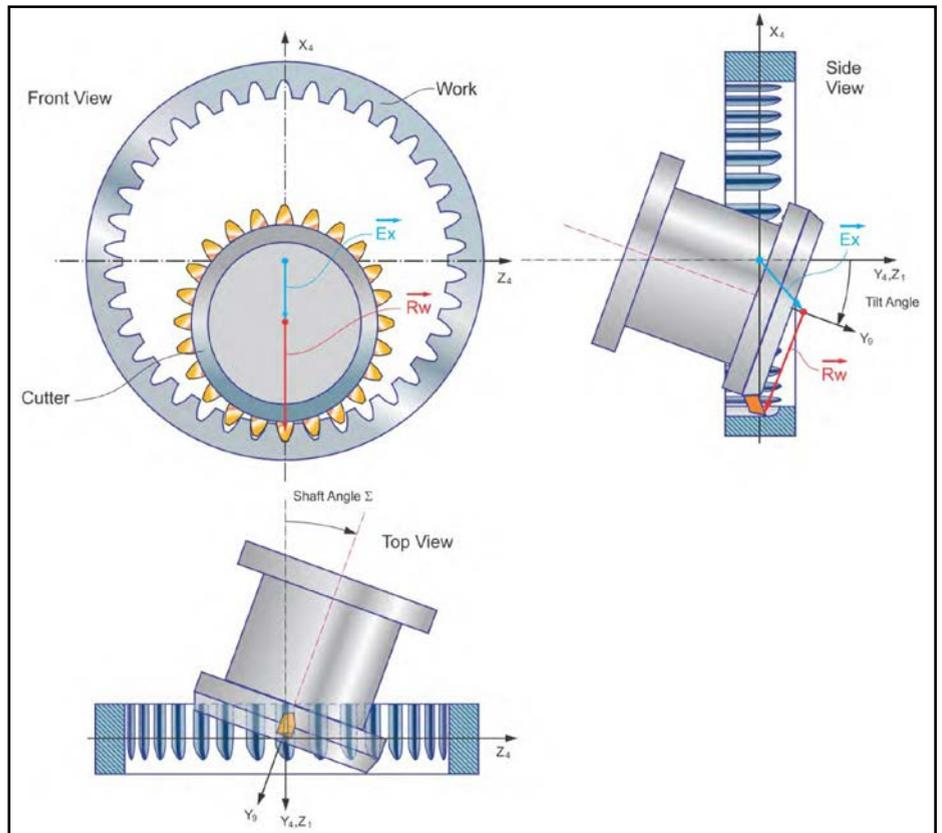
Figure 1 Basic geometry and kinematics of power skiving.
