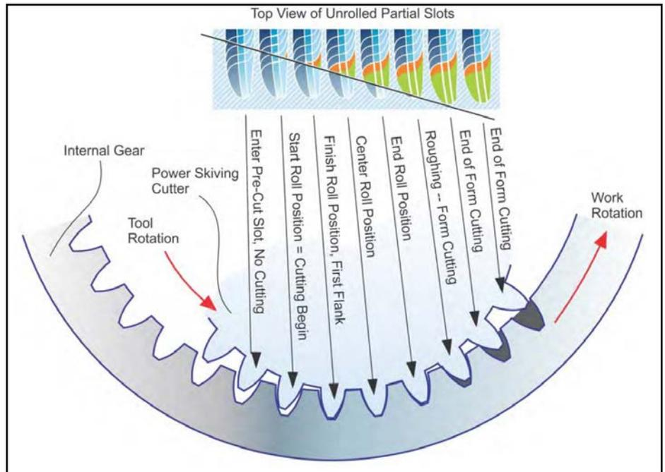
Figure 6 Cutting sequence from engagement to exit.
