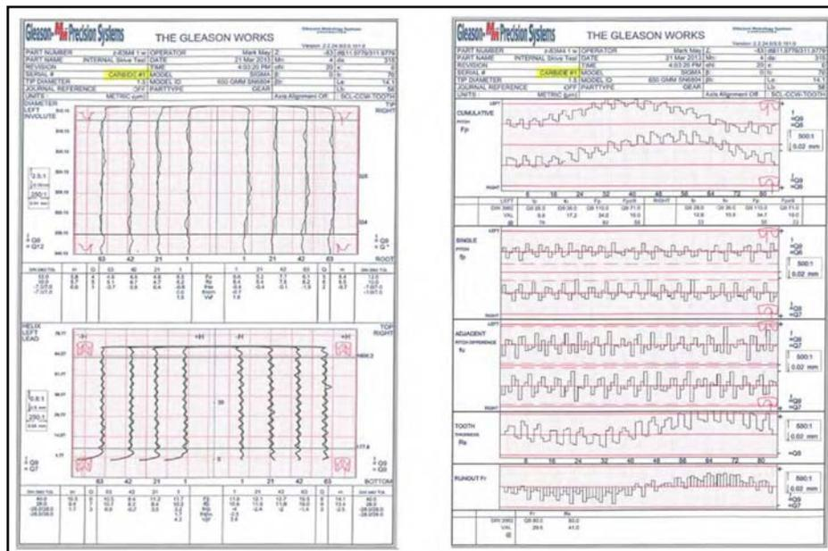
Figure 19 Measurement: profile, lead and spacing.
