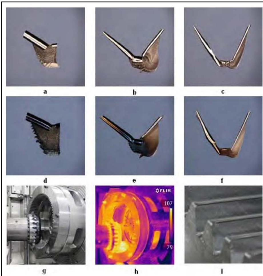
Figure 17 Chips from wet/dry skiving and process temperature.
