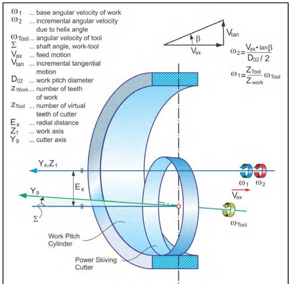
Figure 2 Pitch cylinders of work and tool.
