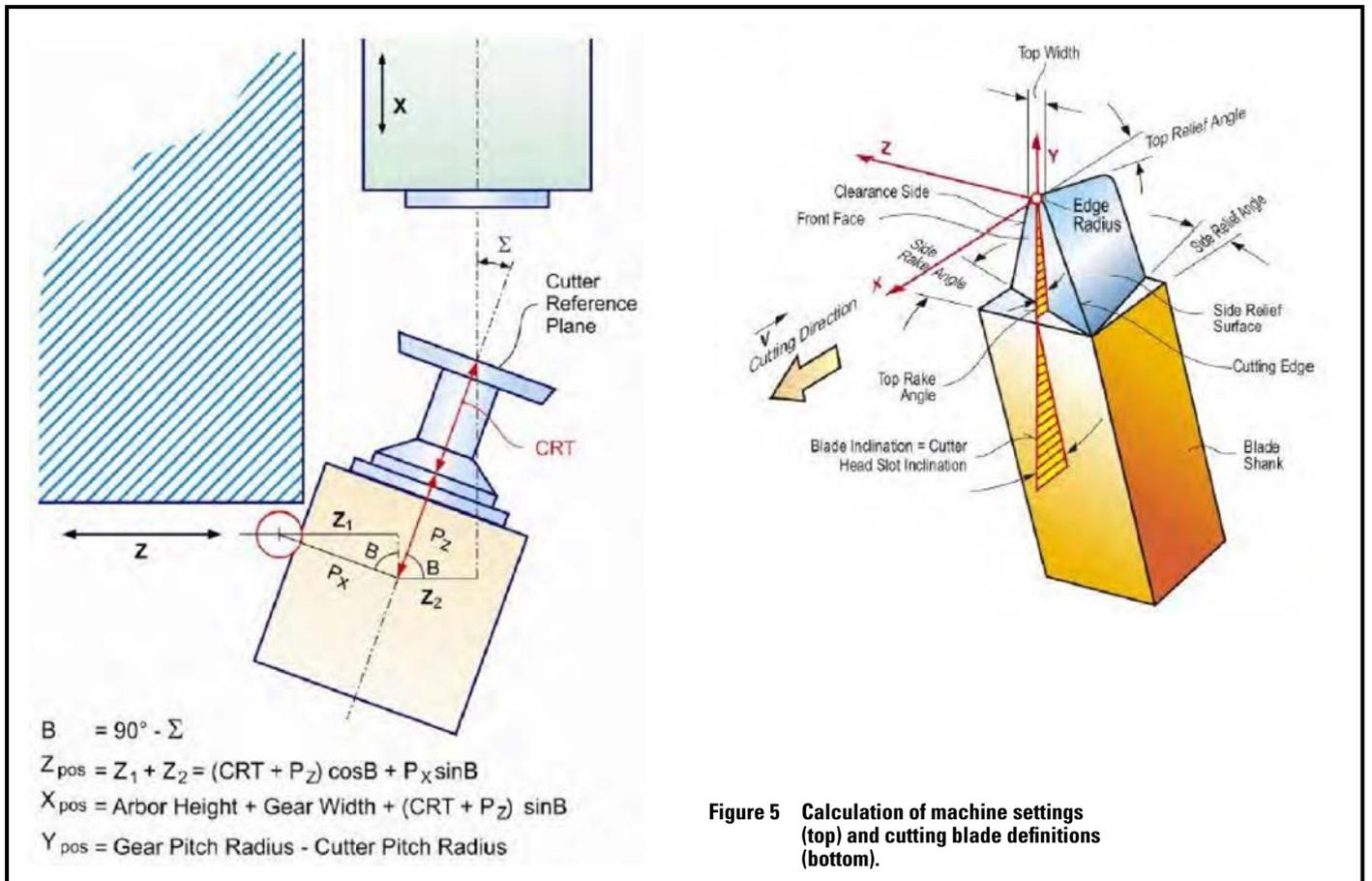
**Figure 5 Calculation of machine settings (top) and cutting blade definitions (bottom).**
