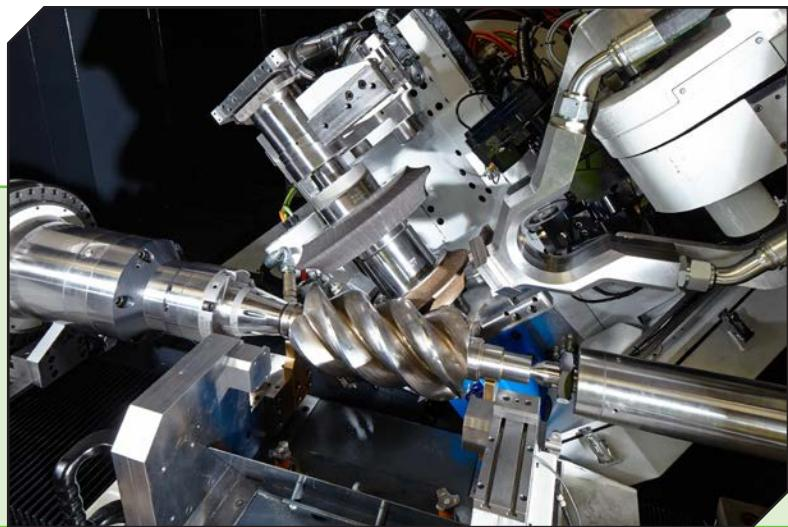
same functions on blanks exceeding one metre diameter. The flexibility of EX series milling machines means that they are equally efficient at producing complex components with helical screw profiles and gear parts such as worm shafts.
