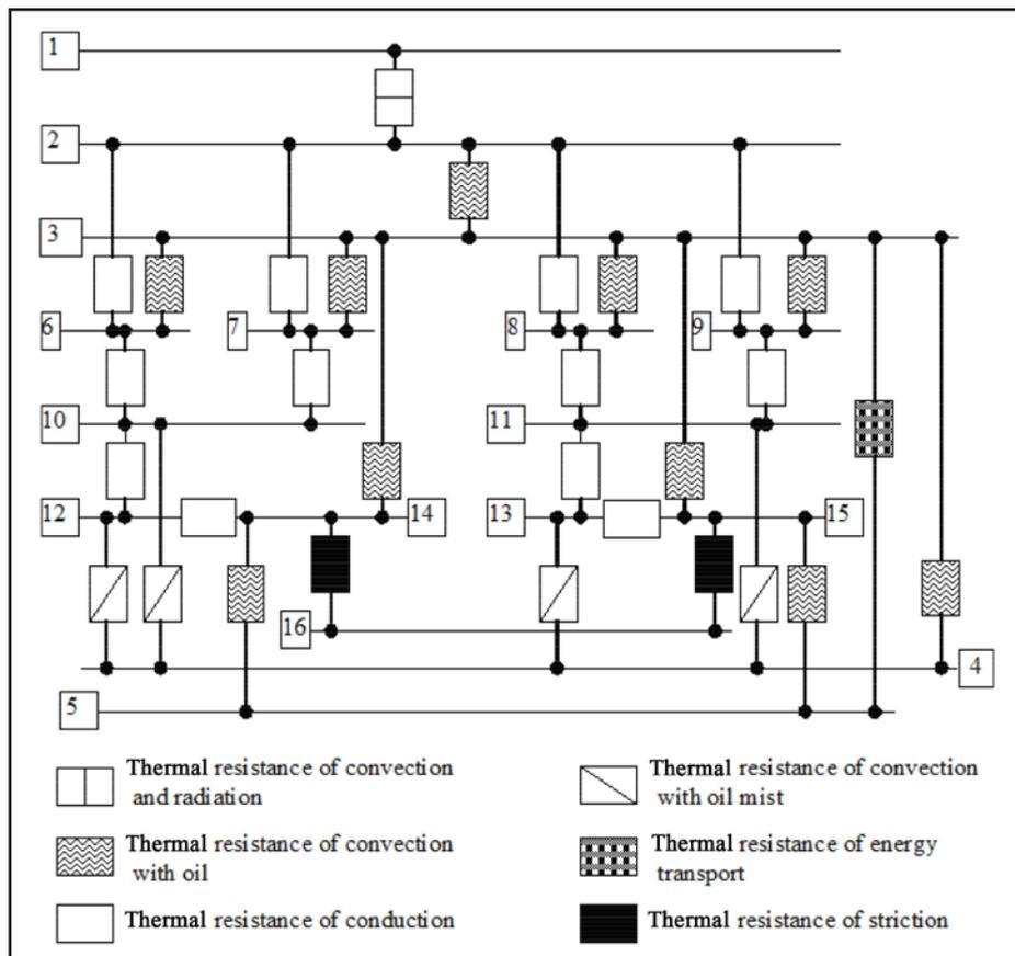
Figure 2 Thermal network of oil jet-lubricated, one-stage gear unit.
