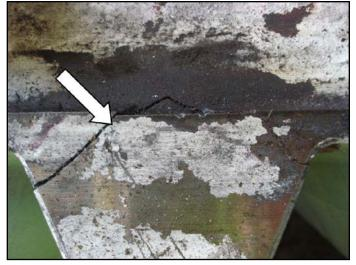
Figure 3 Tooth root crack due to misalignment.
