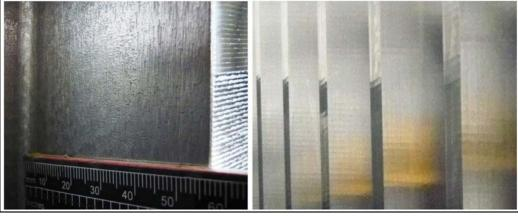
Figure 5 (Left) Surface "scraping" on a tooth flank due to HSS tool wear on a 300 HBW gear: Ra 5 μm; (right) 320 HBW gear cut with carbide tools: Ra 0.6 μm.
