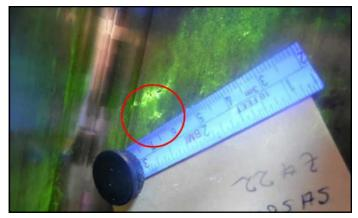
Figure 2 Micro-shrinkage into a cast steel girth gear.
