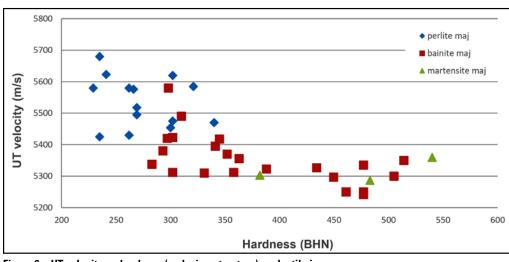
Figure 6 UT velocity vs. hardness (and microstructure) on ductile iron gears.
