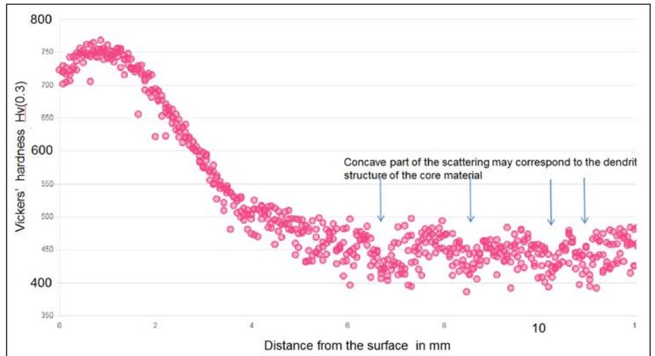
Figure 15 Case hardness of carburized gear tooth.
