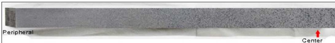
**Figure 6** Macro-etched figure of 500 mm rectangular CrMo steel slab made by rolling.
