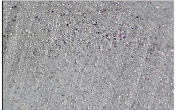
Figure 1 Inclusions that appear on the gear tooth.
