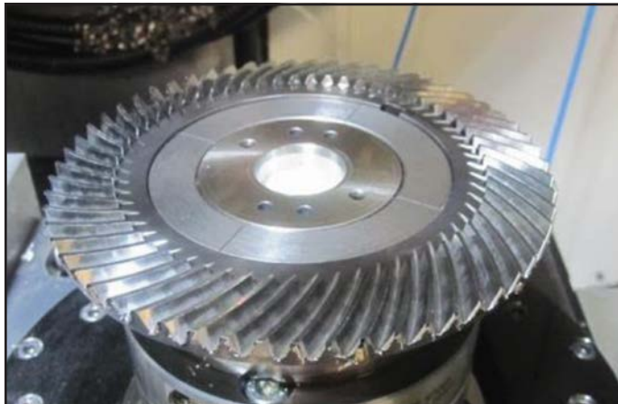
Figure 11 Z=59 gear after soft cut.
