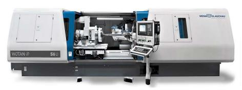
750 mm. Typical workpieces include railway axles, rollers, pipes and shafts.
