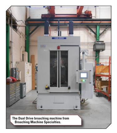
itself is standardized doesn't mean its tooling has to be, as well. Broach tools, fixtures, automation, you name it — the Dual Drive can still mount custom tooling for different jobs, as well as tooling from other manufacturers.
