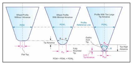
Figure 6 Wheel tip truncation due to tip advance.
