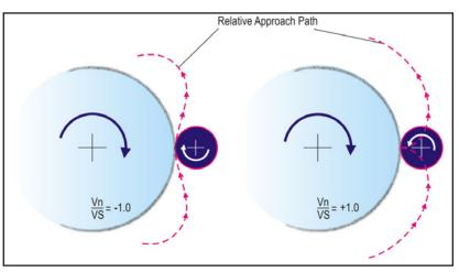
Figure 2 Pure shearing (left) and pure crushing (right).
