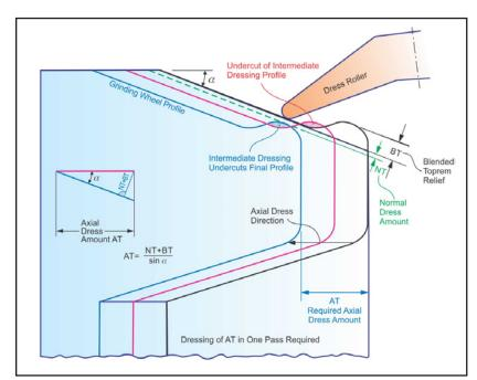
Figure 4 Undercut on grinding wheel profile due to blended toprem.
