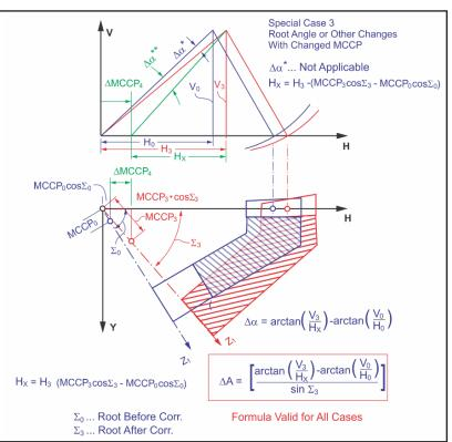
Figure 8 Universal phase angle adjustment.
