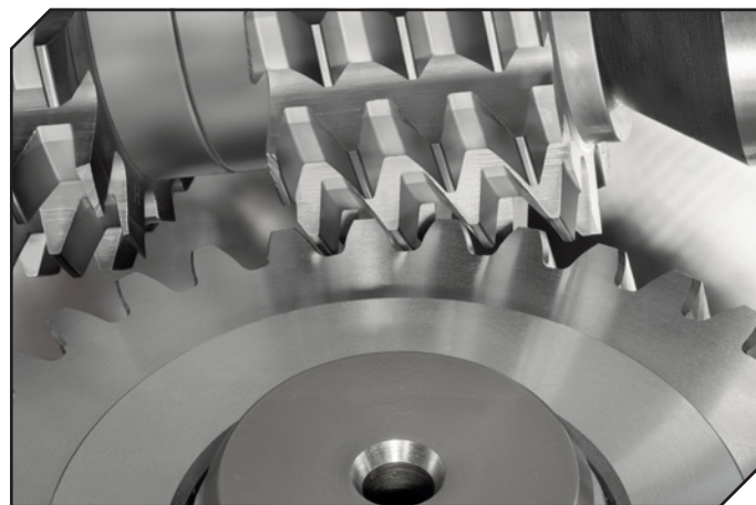
Chamfer hobbing for burr free flanks.
