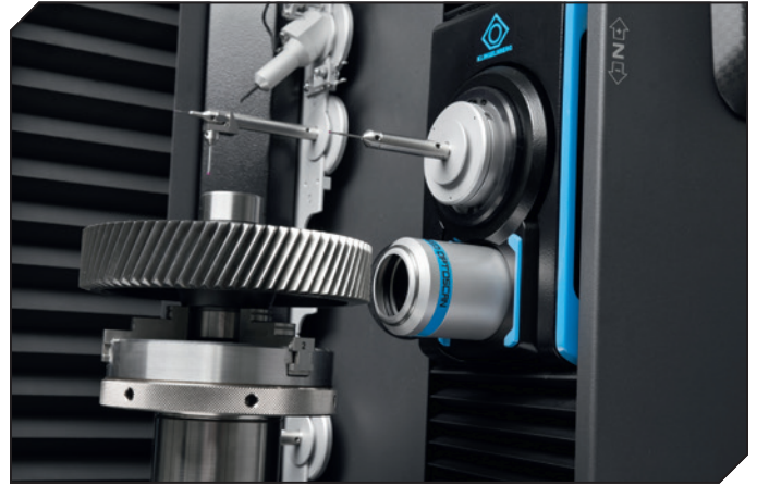
Figure 1 Pitch Measurement with HISPEED OPTOSCAN.
