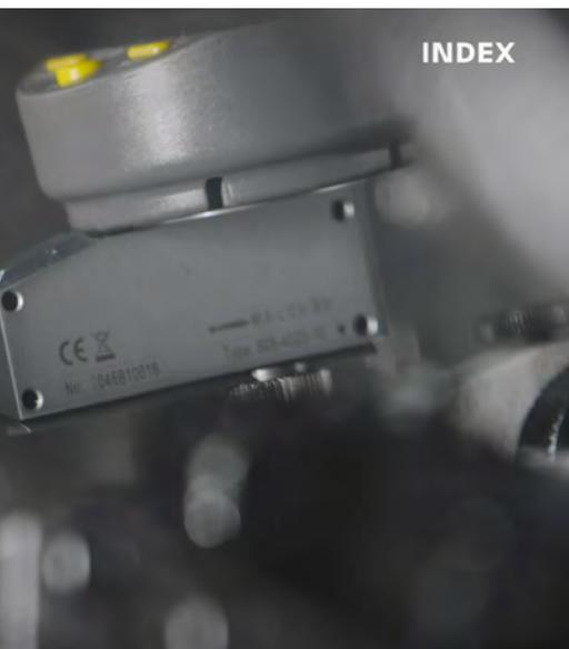
The CenterMaster system allows operators with no specialized knowledge or experience to set up a drill in two to three minutes. Additionally, it provides a repeatable accuracy of <math><5 \mu\text{m}</math>.
