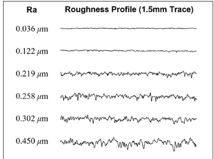
Figure 2—Magnified roughness profiles.
