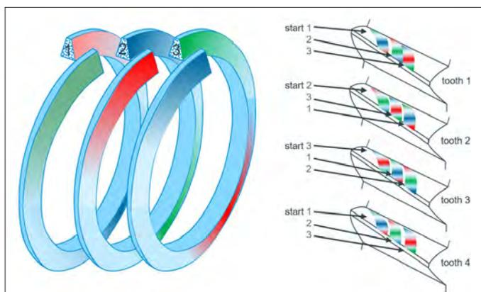
Figure 7—Flank surface modulation.
