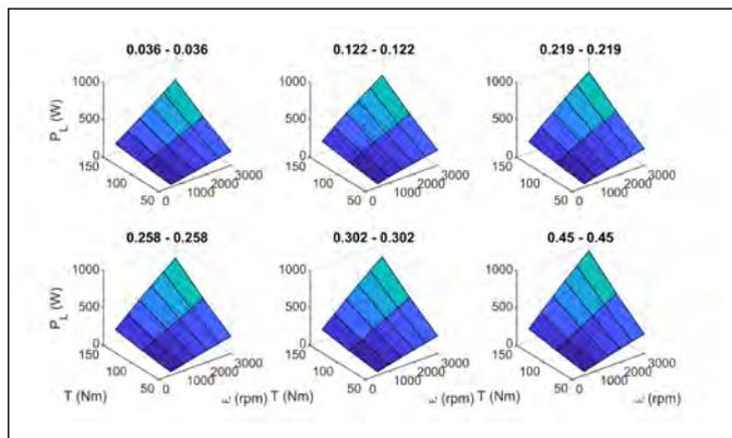
Figure 4—Predicted mechanical power loss for equivalent surface pairings.
