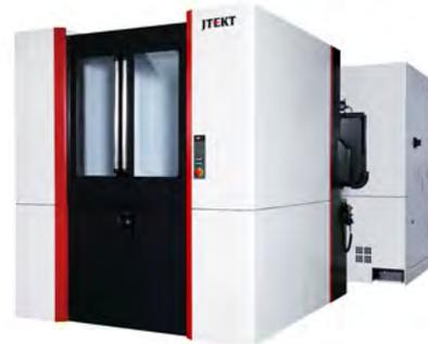
in the FH5000 series are equipped with a 50-taper spindle, 45 tools, and a longer x-axis travel.
