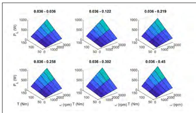
Figure 5—Predicted mechanical power loss for 0036 surface pairings.
