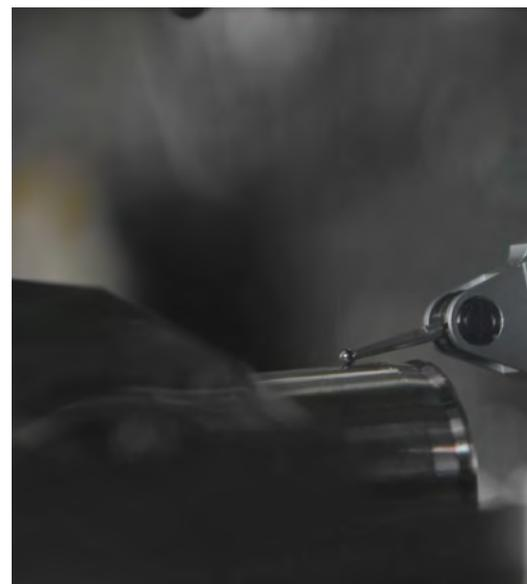
The new HGV water plug machining tool from Ceratizit is available in diameters ranging from 25 to 65 mm. The tool holder is designed and manufactured as a special tool in line with the customer's length and diameter requirements. The indexable inserts for roughing and fine boring are standard stock products.
