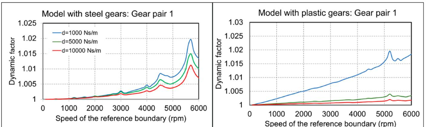
Figure 4—Dynamic factor of the models with different gear meshing damping.
