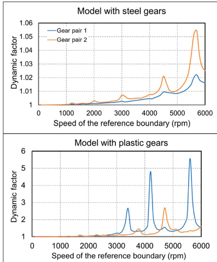
Figure 2—Dynamic factor without gear meshing damping,  $d=0$  Ns/m.
