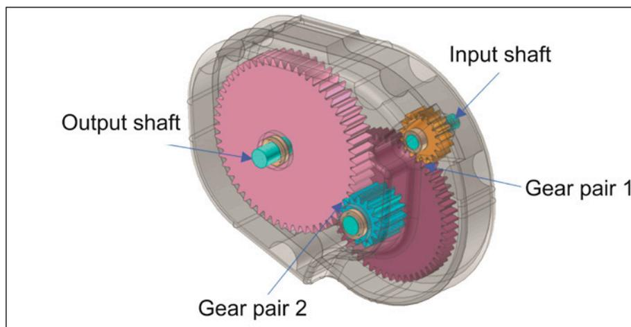
Figure 1—A two-stage gearbox model layout.
