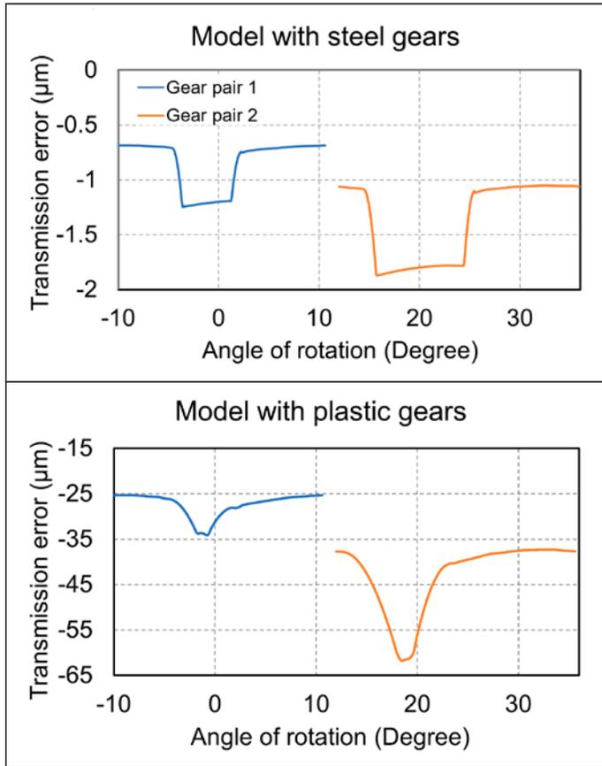
Figure 3—Transmission error of the gear pairs.
