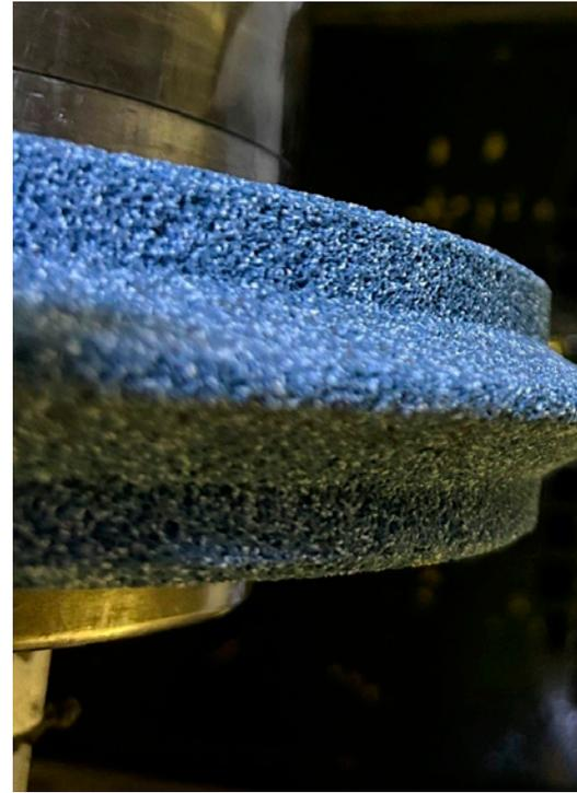
parameters in the profile grinding process can result in increased cycle time, poor gear quality, burning and increased scrap in gear production. Consulting with an application engineer, such as from an abrasives manufacturer like Weiler Abrasives, can improve results.
