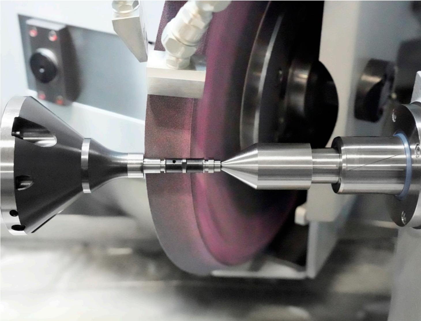
*New manufacturing cell, dedicated to hydraulic workholding, gives Gleason total product quality control throughout the entire value stream. This includes the final hard finish grinding before the workholding is assembled, tested, and inspected.*
