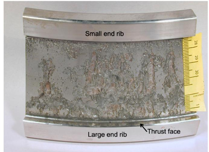
Figure 4—section of the IR with severe macropitting.
