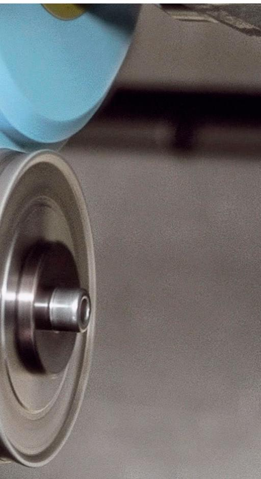
Action of a profile grinding wheel being dressed to demonstrate the method used.
