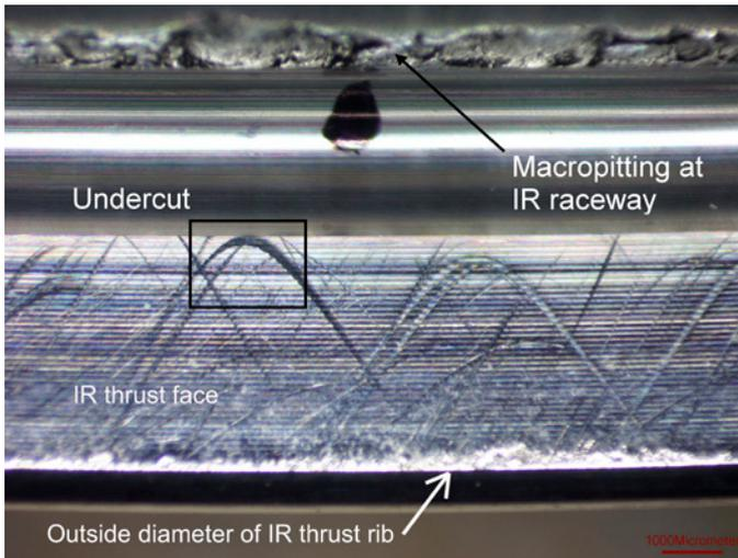
Figure 5—LOM image of the IR thrust rib.
