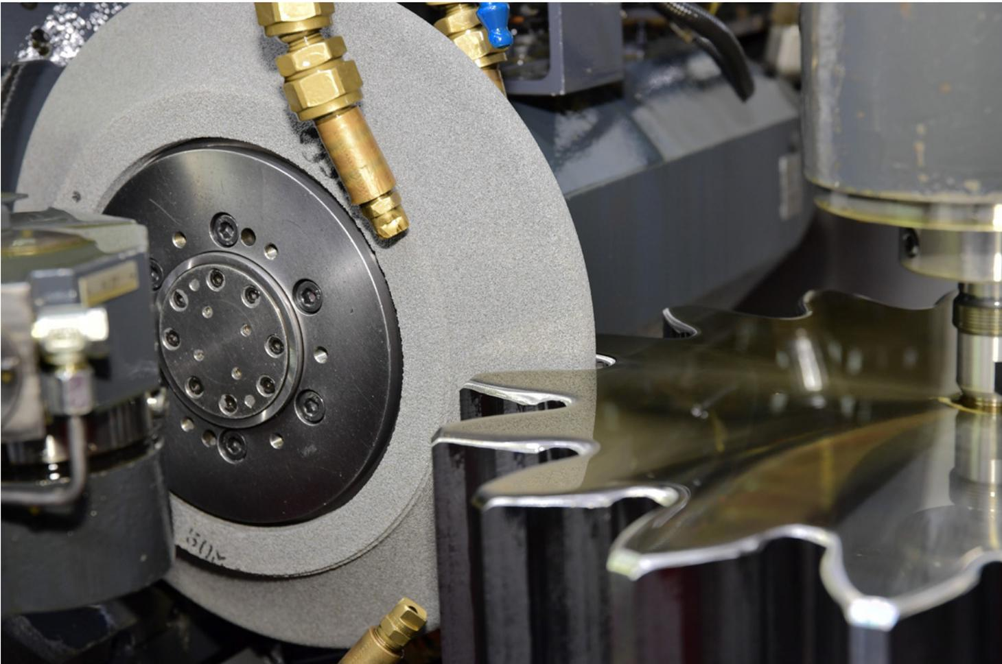
*Profile grinding offers versatility and can be used on gears with clearance issues that do not allow for other grinding processes.*
