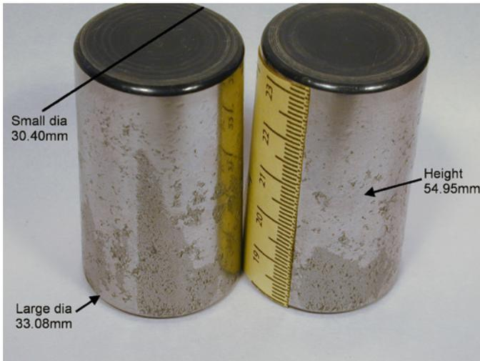
Figure 2—TRB rollers with micropitting toward large ends.
