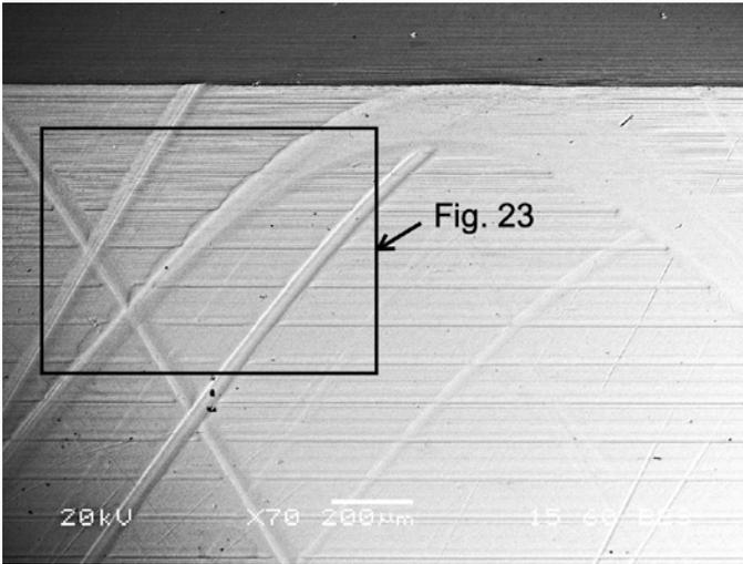
Figure 21—BSE image of the IR thrust rib.
