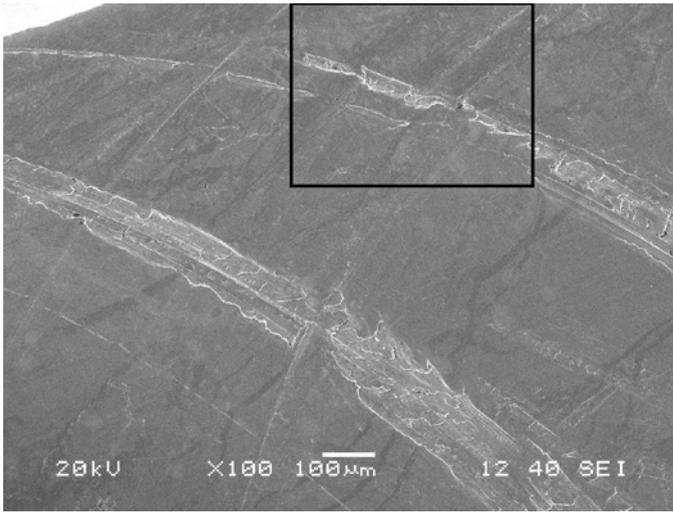
Figure 17—SEM image of roller end at higher magnification.
