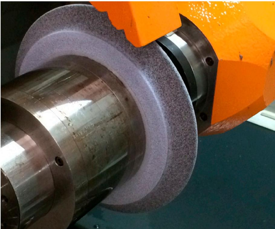
*Profile grinding with the wrong wheel can add considerable cost to an operation. This example shows extreme loading on a profile grinding wheel because it was the wrong wheel choice for the job. Working with an applications engineer can help avoid this issue.*
