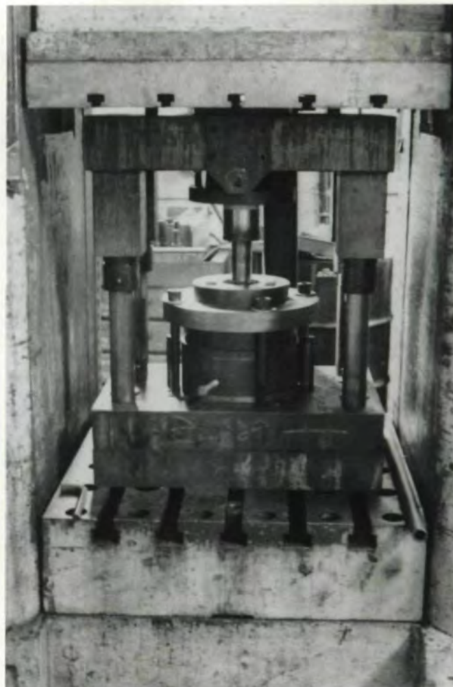
Fig. 11—Tool Setup for Spur Gear Extrusion Trials
