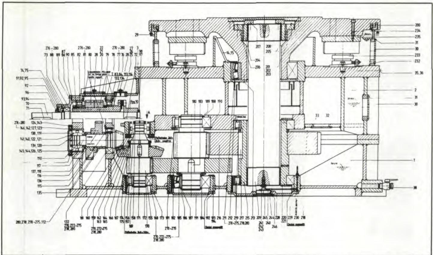
Fig. 7—Rolling mill gear unit with two way power branching (see scheme in Fig. 8). Power  $P = 1350 \text{ kW}$ ; shaft speeds  $n_1 = 980 \text{ min}^{-1}$ ,  $n_2 = 24.5 \text{ min}^{-1}$ . Total weight including flange disk  $G = 82 \text{ t}$ . (Flender-Kienast-Conception)
