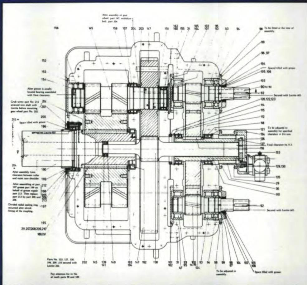
Fig. 9—Tube mill central gear unit with two power branching stages. Transmission power  $P = 4500$  kW; shaft speeds  $n_1 = 490$  min<sup>-1</sup>;  $n_2 = 12.6$  min<sup>-1</sup>; gear unit weight  $G = 100$  t
