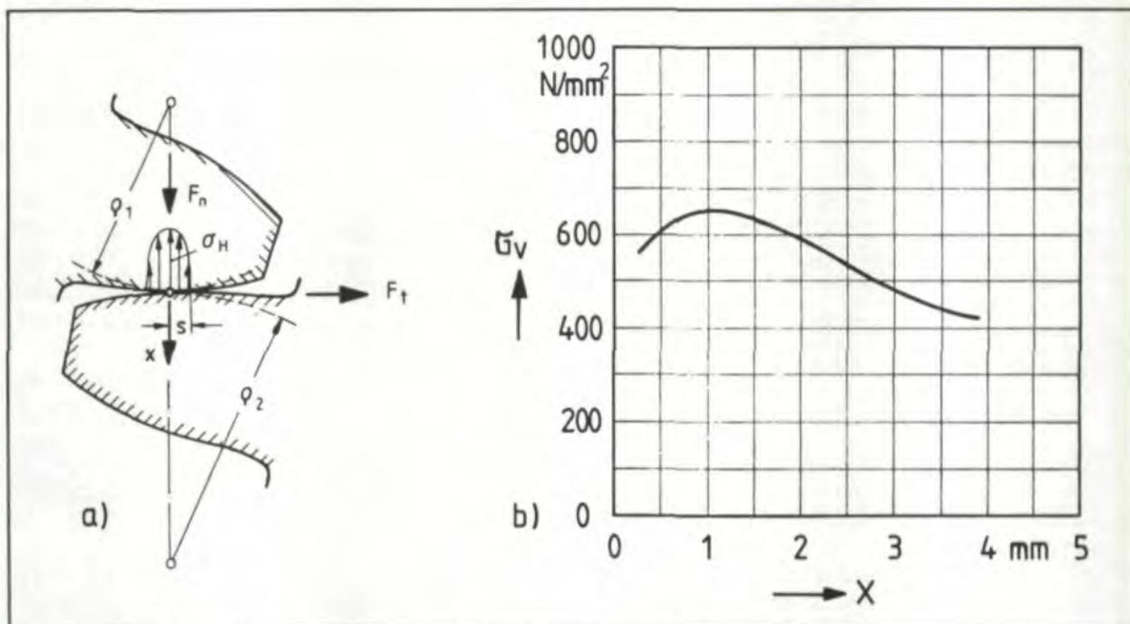
Fig. 1 a) Contact of two tooth flanks.  $\rho_1, \rho_2$  = radii of curvature at the contact point of unloaded flanks;
