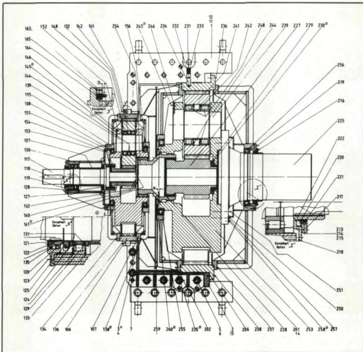
Fig. 10—Two stage planetary gear unit for ball mill drive with three way power branching per stage. Transmission power  $P = 4050 \text{ kW}$ ; shaft speeds  $n_1 = 485 \text{ min}^{-1}$ ;  $n_2 = 13.8 \text{ min}^{-1}$ ; gear unit weight  $G = 72 \text{ t}$
