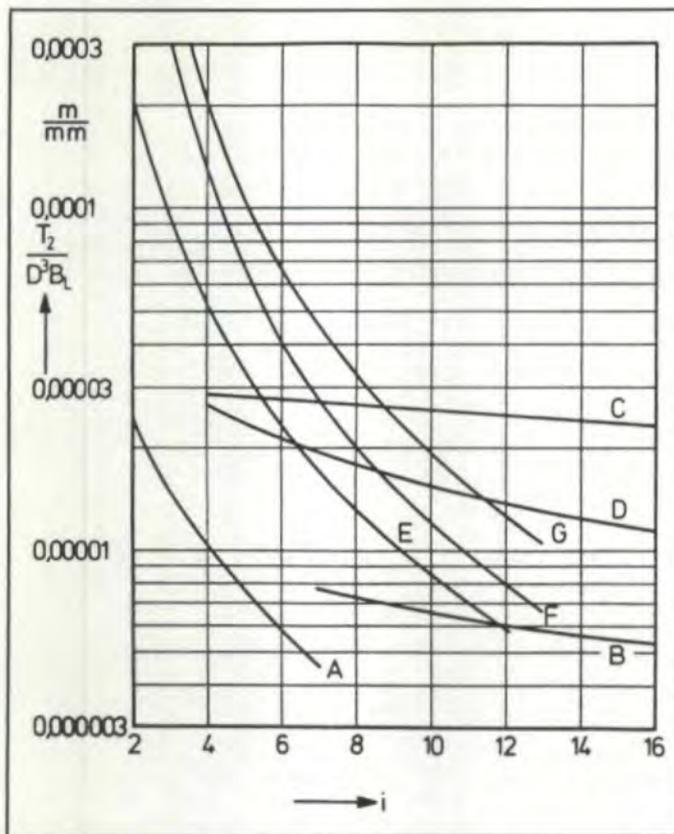
Fig. 4—Dependence of relative (to size) torque of gear units according to Fig. 3 on the transmission ratio  $i$ .  $T_2$  = torque of shaft 2 in Nm;  $D$  = design length or diameter in m;  $B_L$  = load value in  $N/mm^2$
