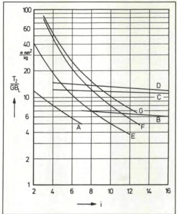
Fig. 5—Dependence of relative (to weight) torque of gear units according to Fig. 3 on the transmission ratio  $i$ .  $T_2$  = torque of shaft 2 in Nm;  $G$  = gear unit weight in kg;  $B_L$  = load value in  $N/mm^2$
