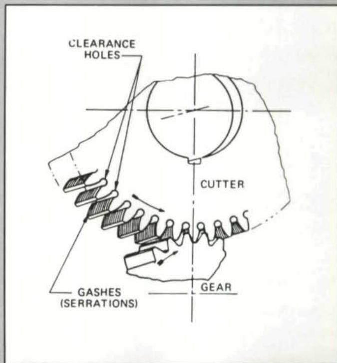
Fig. 1—Work gear in crossed axes mesh with rotary shaving cutter mounted above.
