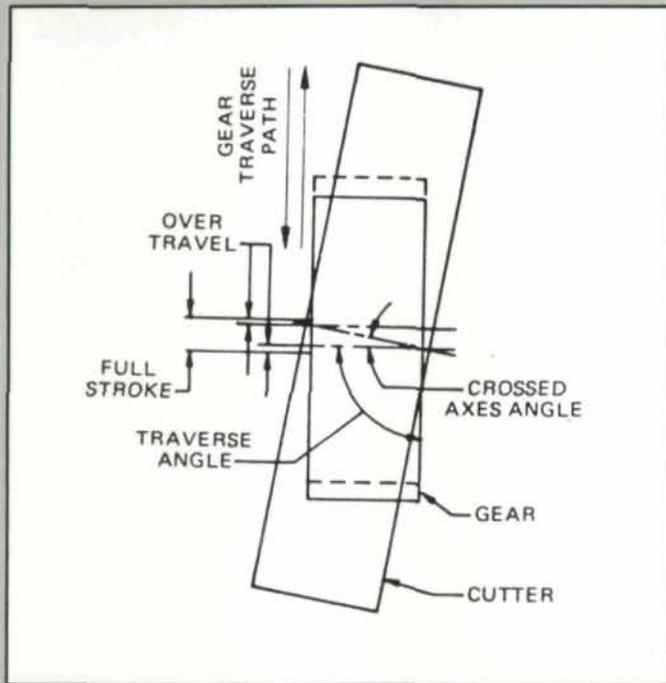
Fig. 8—Tangential shaving (underpass)
