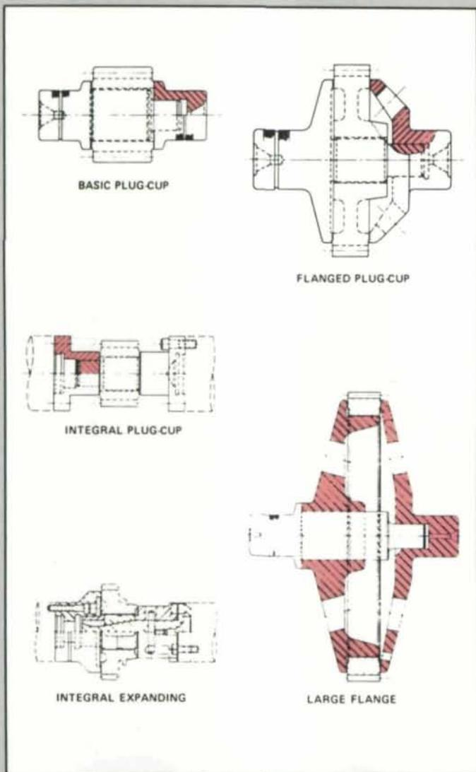
Fig. 10—Typical gear shaving arbors for external gears.
