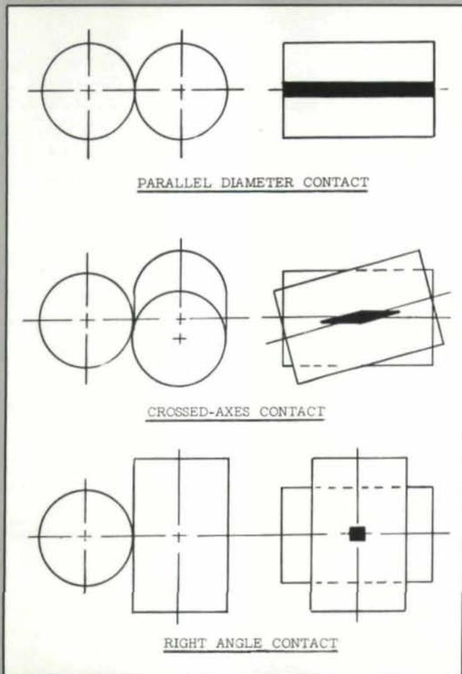
Fig. 3—How the contact between cylinders changes as the angle between their axes is varied.
