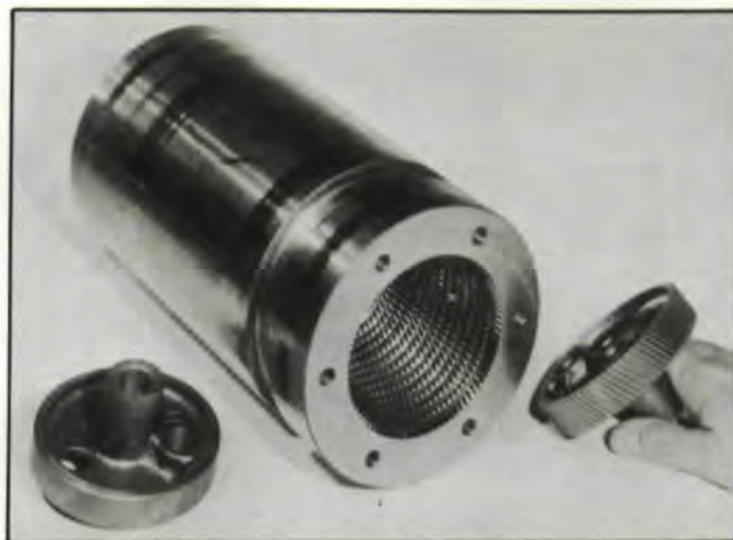
Fig. 17 — A solid HSS pot broaching tool that produces external helical cast iron running gears.
