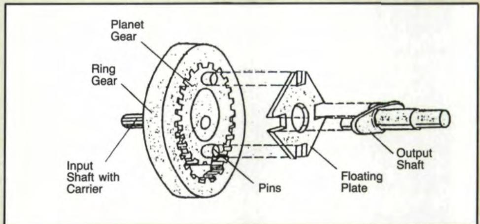
Fig. 2 - KHV with floating plate equal velocity mechanism.
