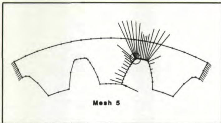
Fig. 7—Stress distribution along the boundary for an internal gear supported at the ends.
