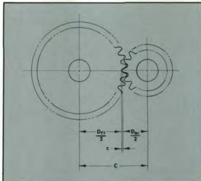
Fig. 2 – Center distance using constant radial clearance.
