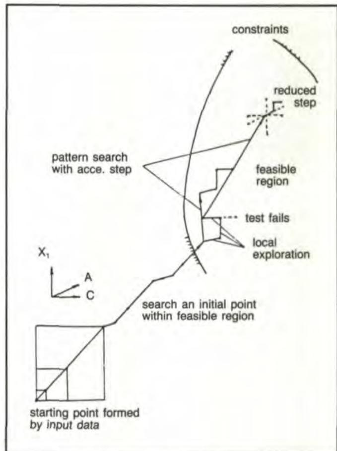
Fig. 3—The process of the optimizing method.
