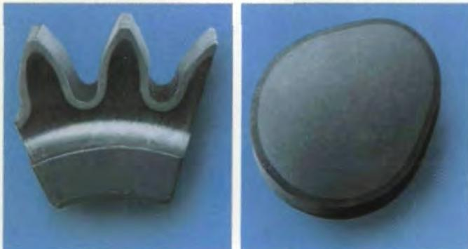
Cross section of camshaft lobe demonstrates uniformity of hardening. Multi-frequency, high intensity hardening of gears produces a high hardness characteristic for improved surface contact fatigue life. High residual compressive stress in the root area is also achieved for improved tooth strength.
