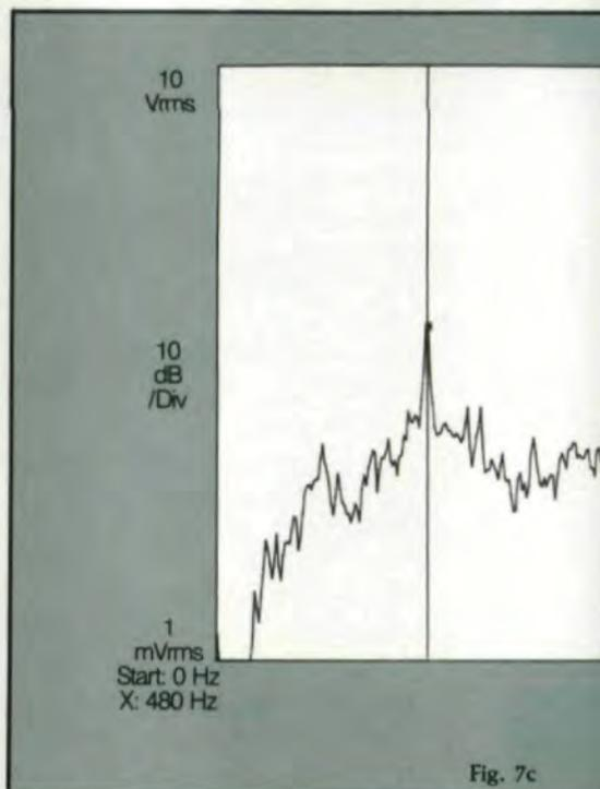
peaks in this display represent the structural resonant frequencies. These frequencies could be excited at any vehicle speed by the appropriate mesh frequency or harmonics that happen to coincide.
