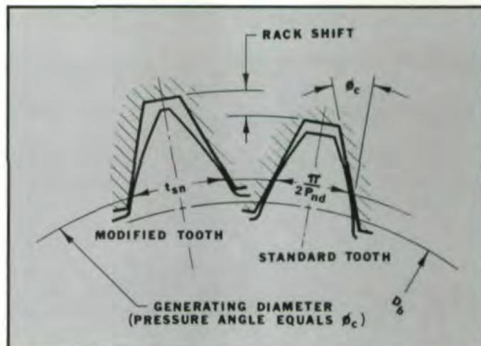
Fig. 4—Addendum modification factor by the tooth thickness method.
