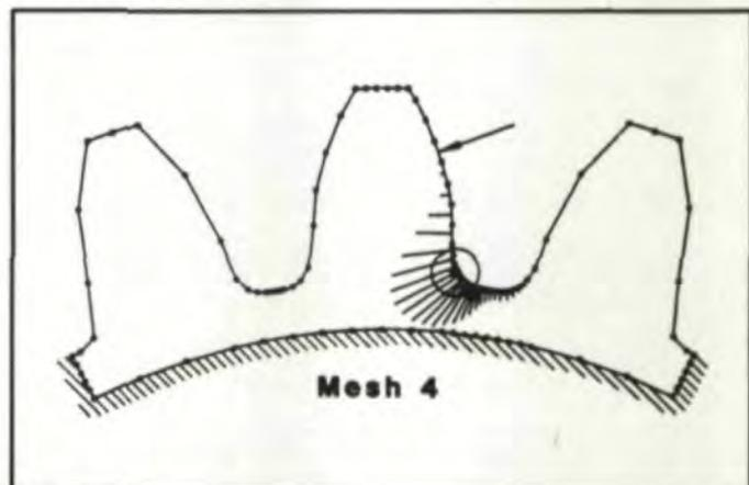
Fig. 6—Stress distribution along the boundary for a thin rimmed external gear supported along the inner bore.
