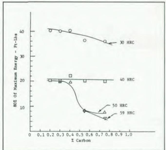
Fig. 10—Isohardness relation of carbon and toughness. Toughness determined by Charpy V-notch.<sup>(10)</sup>
