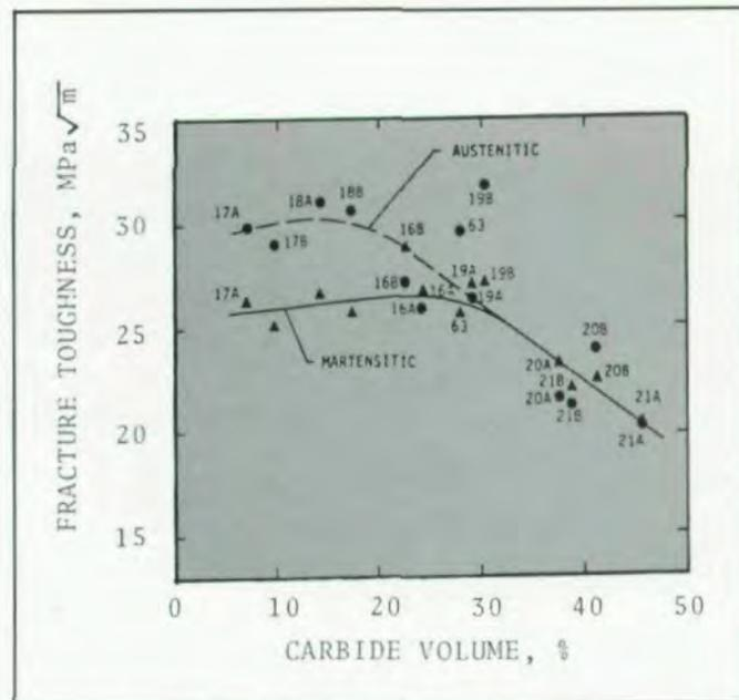
Fig. 8—Influence of carbides on fracture toughness of martensitic and austenitic white cast irons.<sup>(5)</sup>
