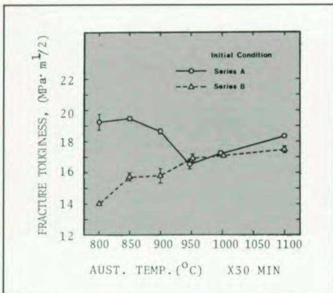
Fig. 3—Influence of starting microstructure on  $K_{IC}$  of 52100 steel. Series A had proeutectoid carbides. Series B contained only fine carbides.<sup>14)</sup>
