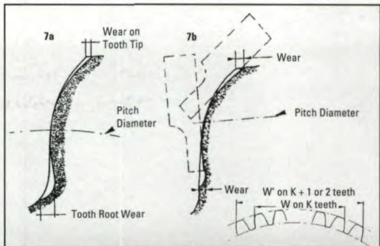
Fig. 7a - Distinctive aspect of distortion of gear teeth profiles under wear action. 7b - Principle of direct wear measurement.
