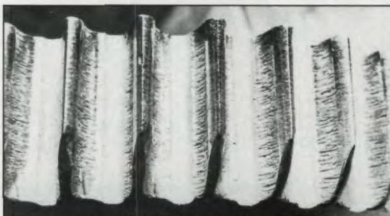
Fig. 4 - Abrasive wear with important loss of material.
