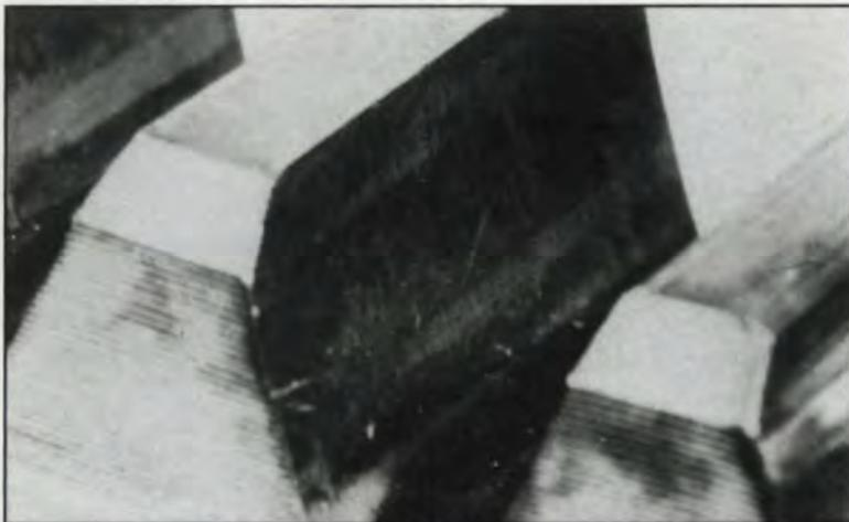
Fig. 9 - Normal wear. Aspect of a large gear wheel flank lubricated with grease.
