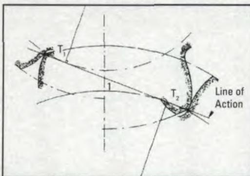
Fig. 5 - Line of action of a cylindrical gear.
