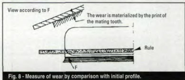
Fig. 8 - Measure of wear by comparison with initial profile.
