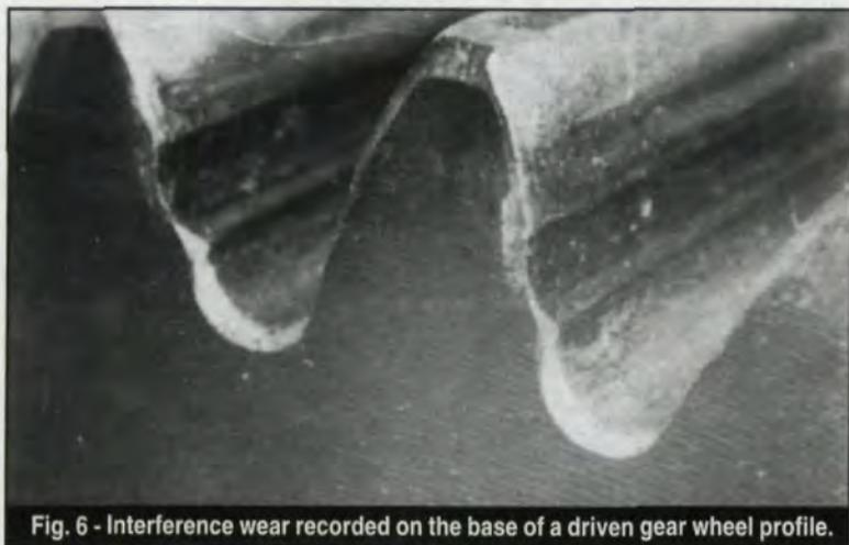
Fig. 6 - Interference wear recorded on the base of a driven gear wheel profile.
