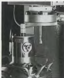
Fig. 30 — Roughing and finishing an internal gear with a disc cutter in a single setup.
