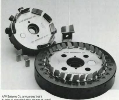
is now a manufacturing source of spiral gear roughing and finishing cutters and bodies
