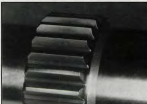
Fig. 15 — Spline end of 9310 multi-metal demonstration sun gear.
