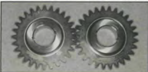
Fig. 10 — Pair of multi-metal fatigue test gears.
