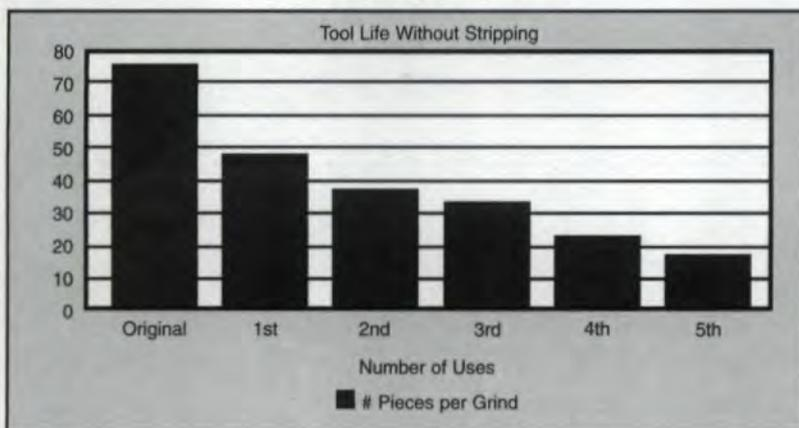
Fig. 2 — Number of pieces produced with recoated TiN shaper cutters.
