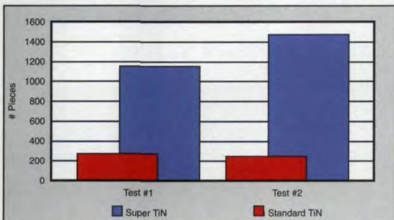
Fig. 7 — Super TiN performance tests at Land Rover.
